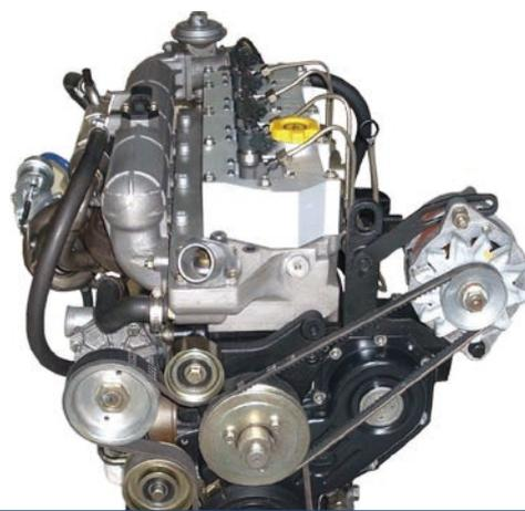
Da-Yeh university advanced vehicle technology research center (AVTRC) is a pioneer in advanced diesel engine development in Taiwan. AVTRC developed a 2.5-liter, direct fuel injection diesel engine to power vehicles, forklifts, and electric generators.
